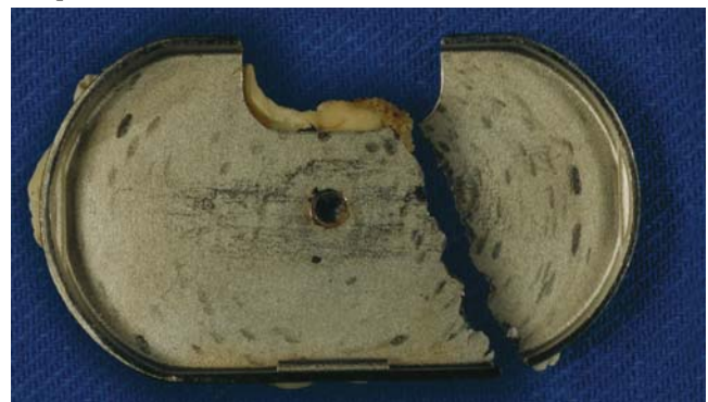
FIGURE 2-12. Visualization of adhesive film transfer demonstrating UHMWPE insert rotatory micromotion in a modular tibial component.
