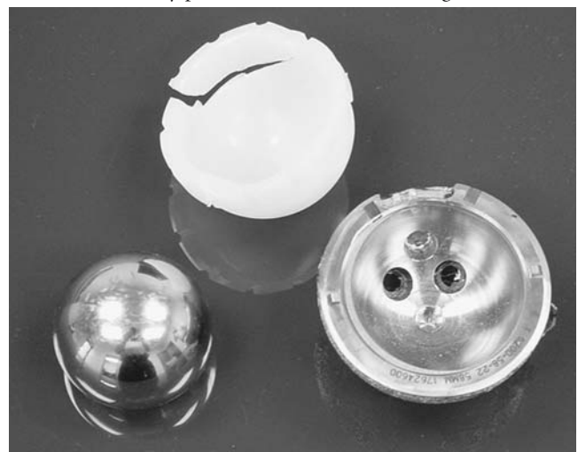
FIGURE 2-21. A 10-month highly cross-linked UHMWPE, revision acetabular liner demonstrating crack initiation and propagation. The decision to retain the acetabular shell in an almost vertical and anteverted position contributed to this early failure, which was compounded by the decision to use a 40-mm femoral head and a correspondingly thin liner. (From Halley, Glassman, Crowninshield 130 by permission of J Bone Joint Surg .)
