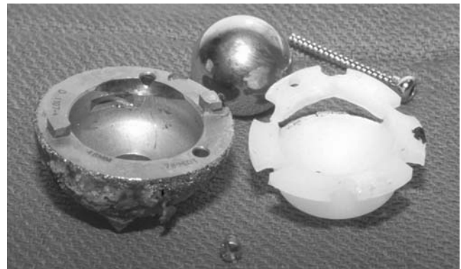
FIGURE 2-20. A 1-year conventional UHMWPE, primary acetabular liner demonstrating crack initiation and propagation. Failure initiated at a sharp edge of a locking point. (From Tradonsky, Postak, Froimson 129 by permission of Clin Orthop .)
