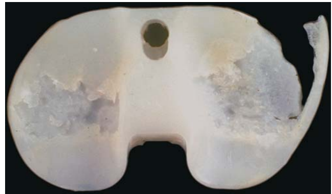
FIGURE 2-3. Six-year retrieval of a heat-pressed tibial component associated with polyethylene fatigue and early delamination.
