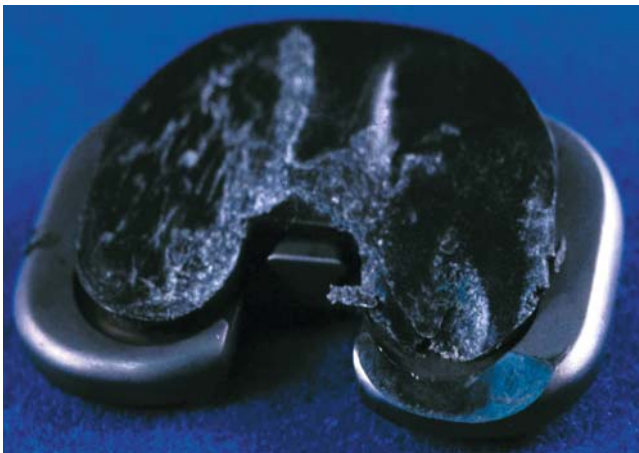
FIGURE 2-1. Five-year retrieval of a failed Poly-2 tibial insert demonstrating a high component wear rate with infiltration of carbon fibers and polyethylene debris into surrounding tissue.
