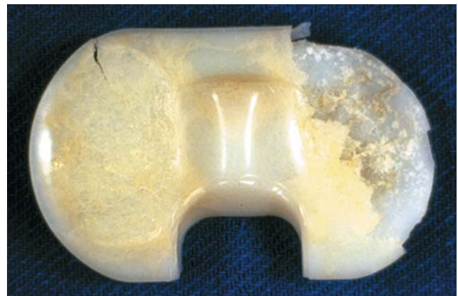
FIGURE 2-5. A Group 2 plateau implanted after 7.6 years of shelf storage and retrieved 3.8 years after implantation. Gross delamination and pitting, characteristics of fatigue failure, are observed. (From Bohl, Bohl, Postak, et al. 34 by permission of Clin Orthop. )
